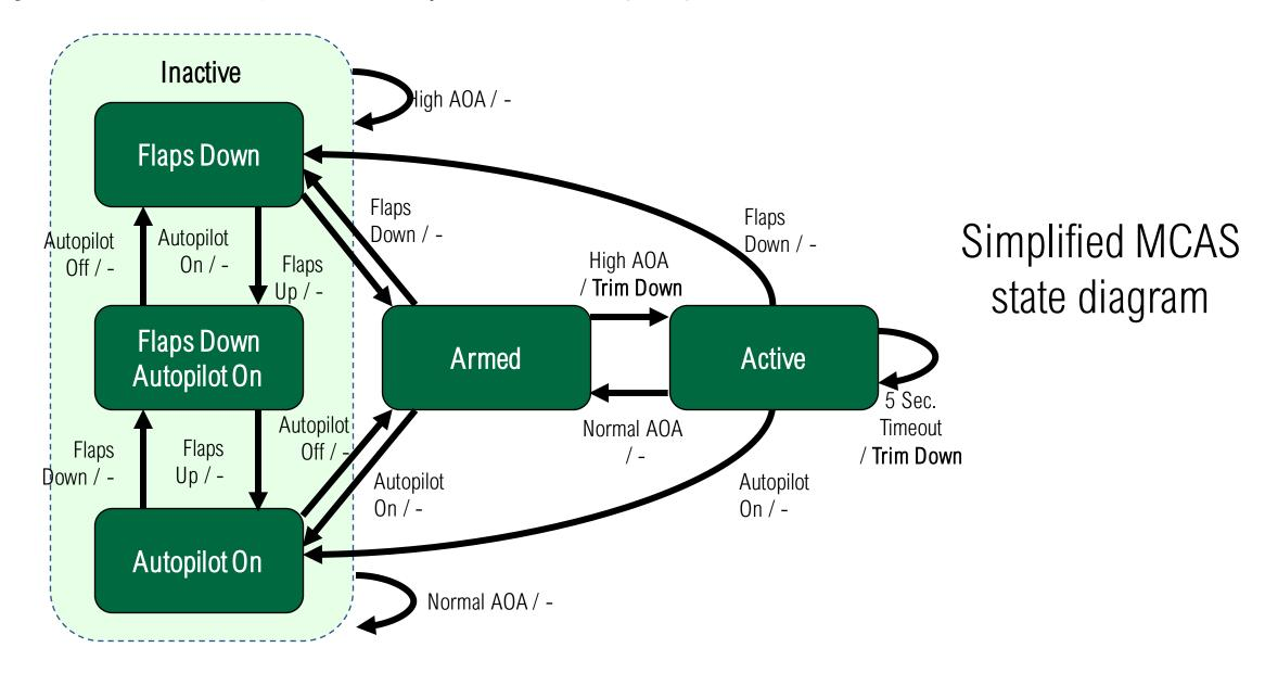
Using the Gherkin system test language, design a system test to verify that MCAS activates (that is, produces a trim-down input) as desired
